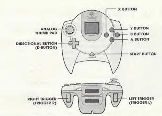
Never touch the Analog Thumb Pad or Triggers L/R while turning the Sega Dreamcast power ON. Doing so may disrupt the controller initialization procedure and result in malfunction. Operation with incompatible controllers is not guaranteed.
